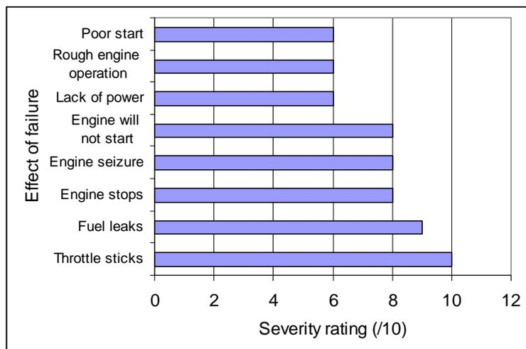
**Figure 7 Severity rating of the effect of failure for components exposed to E20**
