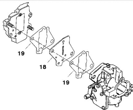
Figure 16 Carburettor and reed assembly
