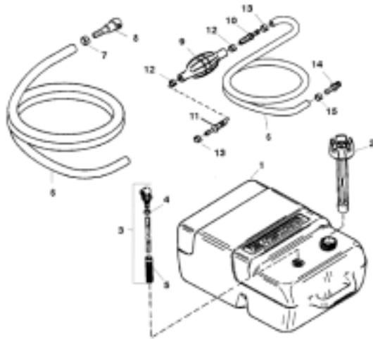
Figure 14 Fuel tank assembly
