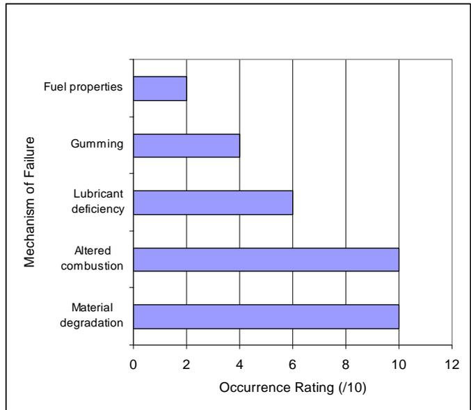
**Figure 9 Occurrence rating for the cause of components exposed to ethanol-blended fuels**
