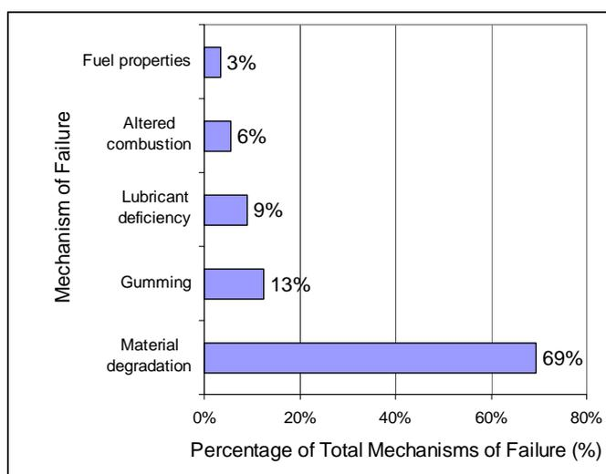
Figure 8 Mechanism of failure vs. Percentage of total
