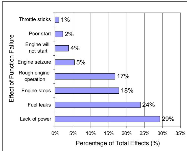
**Figure 6 Effect of component function failure on engine**
