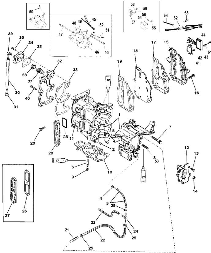
**Figure 18 Cylinder block assembly**
