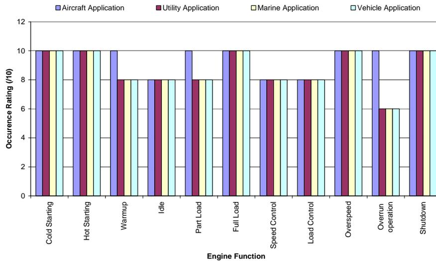
**Figure 3 Occurrence rating for engine function and engine groups**
