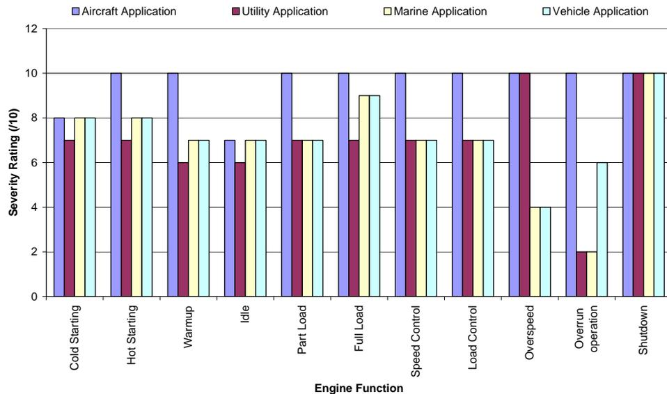
Figure 1 Severity rating for each function and engine group
