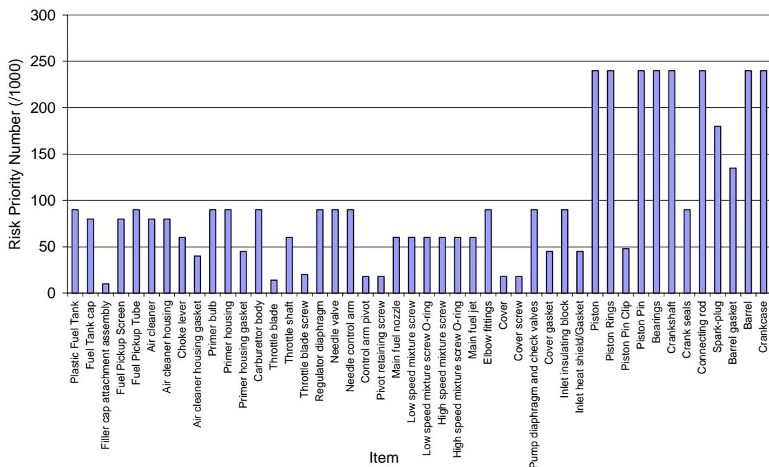
Figure 13 Risk Priority Number for components of FS45 Line-trimmer engine
