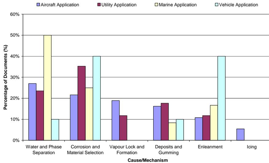
**Figure 2 Results of document search on failure mechanisms**
